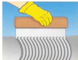
Spreading of Sikafloor®-262 AS N with notched trowel. E.g. Polyplan notched trowel 5/7 mm.
