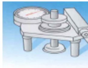
Testing of the substrate Pull-off strength > 1.5 N/mm 2 . E.g. Proceq, Dyna pull-off tester.
