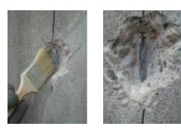
Clean the dust completely from the concrete surface using the brush, or a blower. The surface should be completely free from all loose particles. Improper cleaning results in incorrect measurements of carbonation depths!
