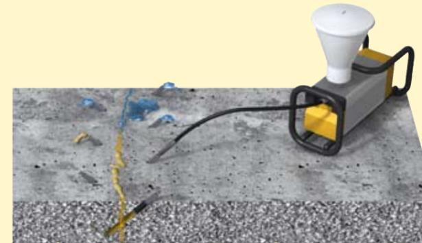
4. When the injection material flows out of the second packer during the injection process, fix the non-return valve on it as quick as possible. Stop injection at the first packer and continue at the second packer.
