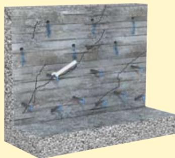
2. Install the mechanical packers. Tighten the mechanical packers so that they can withstand the maximum injection pressures.
