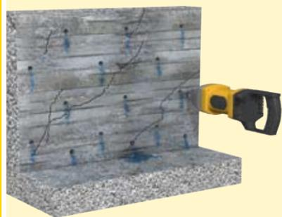
1. Drill holes for the mechanical packers through the leaking building component at a distance of 30–50 cm apart as shown in the figure.
