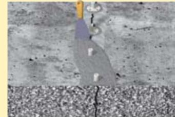
3. Patch the surface of the crack with **Sika® Injection-490**. Ensure that the packer and the crack on the surface are fully covered by the adhesive filler.
