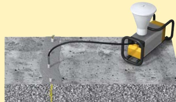
4. As soon as the adhesive has cured, remove the nail and fix the button head fittings (non-return) on the first packer and start the injection process.
