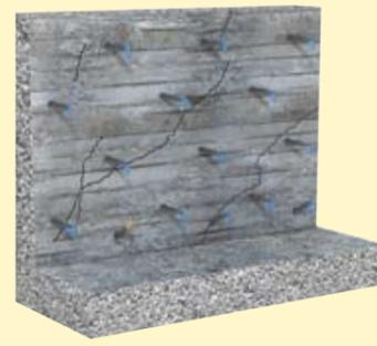
3. Fix the button head (non-return) fittings on the first packer and start the injection process at the lowest row of drill holes.
