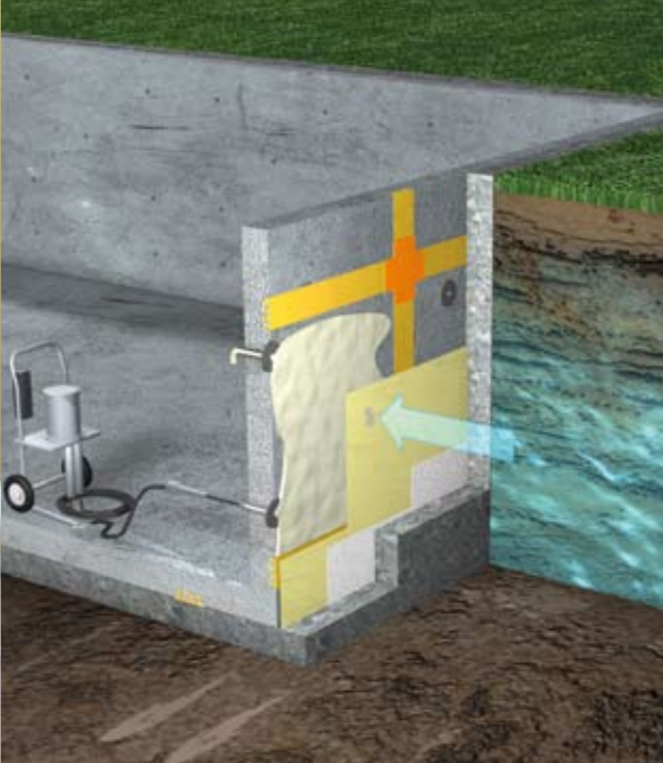
Repairing the waterproofing by the injection of Sika® Injection-305 resin through the Sika® Control pipe and injection port.
