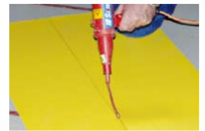
Electric testing with a "holiday" detector
