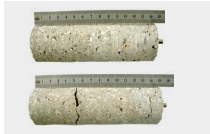
Fig. 8.4.1: Concrete deterioration due to sulfate attack before and after the load shows a strong increase in length because of the spalling attack. First cracks have appeared in sample.
