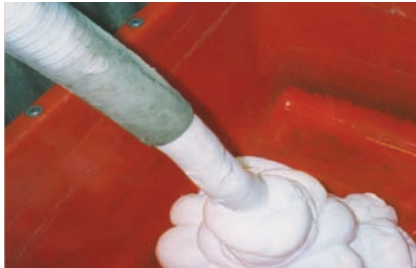
Fig. 8.15.2: Expansion causing additives (e.g. powdered aluminium) are mixed with the mortar for porous concrete. Porous concrete is generally produced industrially. Porous concrete is not really a concrete, it is really a porous mortar.
