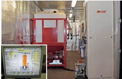
Fig. 8.13.2: Colored concrete demands far more than just adding the pigments. From planning to installation, essential decisions must be made for the application to succeed and the most diverse production steps must be checked and executed expertly. All participants are challenged. Exclusive Color Select® PC Liquid Dispensing System.
