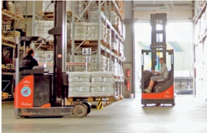
Fig. 8.7.4: Industrial flooring surfaces also experience strong abrasion due to constantly rolling and striking loads in the same places. Hard concrete coatings and special dispersants can enhance the flooring grip and minimize wear.
