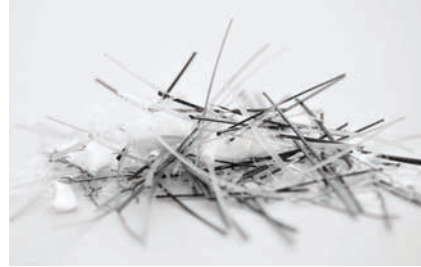
Fig. 8.11.1: Fibers for use in concrete are produced from different materials and qualities of these materials, plus they can have different geometric dimensions and form, according to the required performance of the fresh or hardened concrete.
