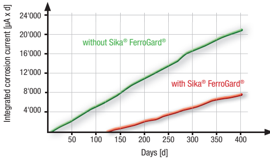
Fig. 8.2.3: The Sika Research Department in Zurich tested the anticorrosive effect of Sika® FerroGard® on cracked concrete beams.
