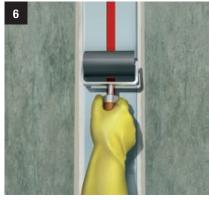
Press the **Sikadur-Combiflex**<sup> $\circ$ </sup> **SG** tape without trapping air into the adhesive by using a suitable roller. The adhesive should be squeezed out on both sides by ~ 5 mm.
