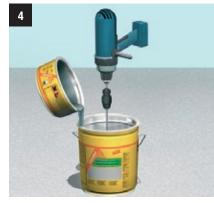
Mix **Sikadur<sup>®</sup>-Combiflex<sup>®</sup> CF** adhesive components A and B for a minimum of 3 minutes until the mix is homogeneous.
