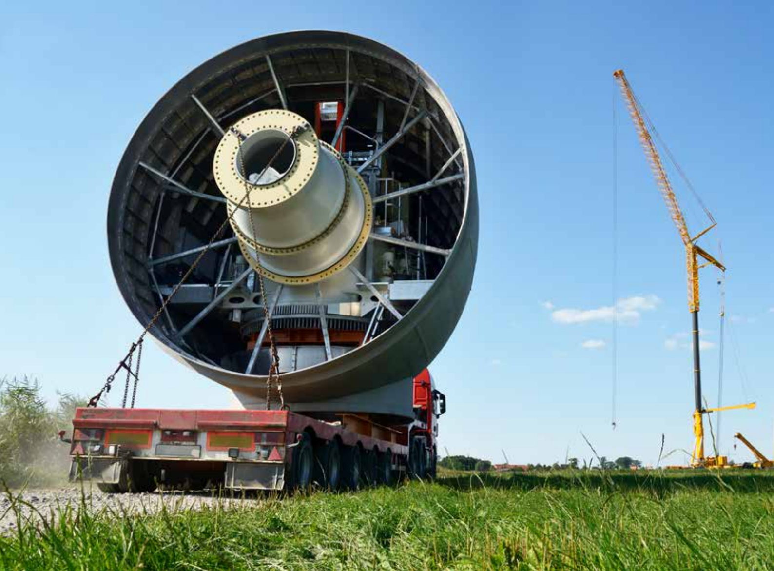
Hub transport to the erection site of the turbine.
