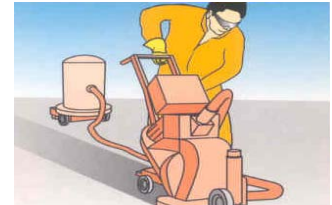
Preparation of the substrate: Blast cleaning or other mechanical means. E.g. Blastrac.
