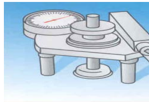
Testing of the substrate Pull-off strength > 1.5 N/mm 2 . E.g. Proceq, Dyna pull-off tester.
