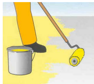
Even application of Primer coat: Sikafloor®-264 with medium to long haired roller or brush. E.g. Polyplan roller and brush.
