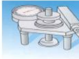
Testing of the substrate Pull-off strength > 1.5 N/mm 2 . E.g. Proceq, Dyna pull-off tester.
