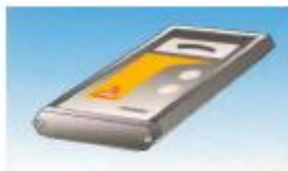
Measuring of the substrate moisture: Moisture content < 4% by weight. E.g. Sika Tramex moisture meter.
