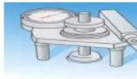
Testing of the substrate Pull-off strength > 1.5 N/mm 2 . E.g. Proceq, Dyna pull-off tester.
