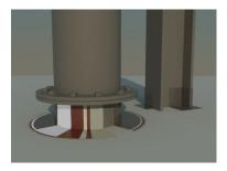
Build up: Sikalastic -601 BC applied in 1 coat, reinforced with Sika® Reemat
