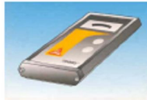
Measuring of the substrate moisture: Moisture content < 4% by weight. E.g. Sika Tramex moisture meter.
