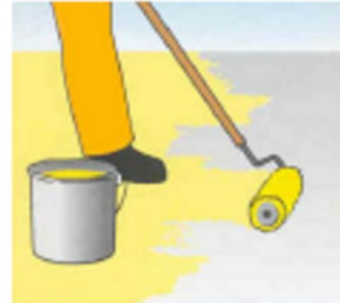
Even application of Primer coat: Sikafloor®-161 with medium to long haired roller or brush. E.g. Polyplan roller and brush.
