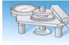
Testing of the substrate Pull-off strength > 1.5 N/mm 2 . E.g. Proceq, Dyna pull-off tester.
