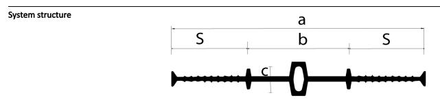
Total width (mm) Width of move- Thickness (mm) c Width of a ment part (mm) b sealing part (mm) D24 (240mm) 85 mm 4.0 mm 77.5 mm
