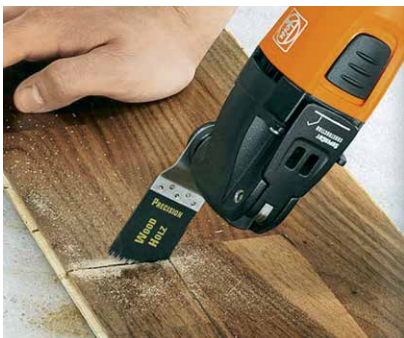
Fig. 48 Cutting planks with vibrating knife
