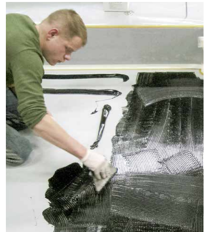
Fig. 55 Application of Sikaflex®-298
