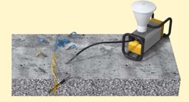
4. When the injection material flows out of the second packer during the injection process, fix the non-return valve on it as quick as possible. Stop injection at the first packer and continue at the second packer.
