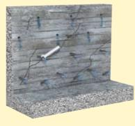
Install the mechanical packers. Tighten the mechanical packers so that they can withstand the maximum injection pressures.
