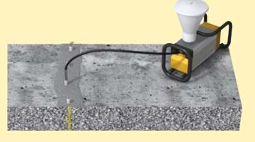
As soon as the adhesive has cured, remove the nail and fix the button head fittings (non-return) on the first packer and start the injection process.
