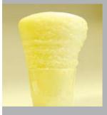
The free expansion rate of **Sika**® **Injection-101** is up to 40 times.
